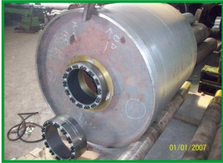
CONVEYOR PULLEY WITH RING FEEDER
